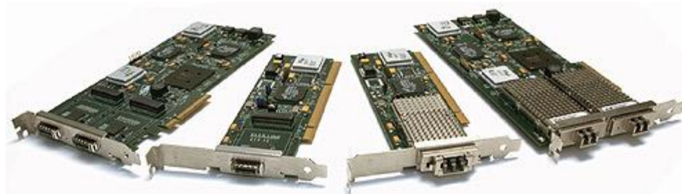
Figure 1. Single and Dual-Port 10Gb/s NIC Adapter Cards
